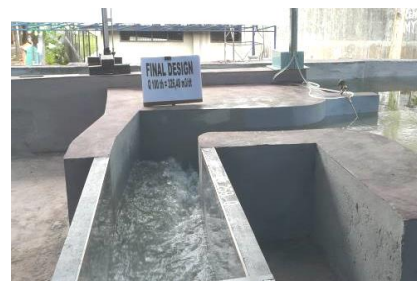
Gambar 15. Model Seri II perubahan dinding approach channel
